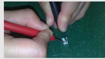
2. The evaporator temperature sensor malfunction (E3)
