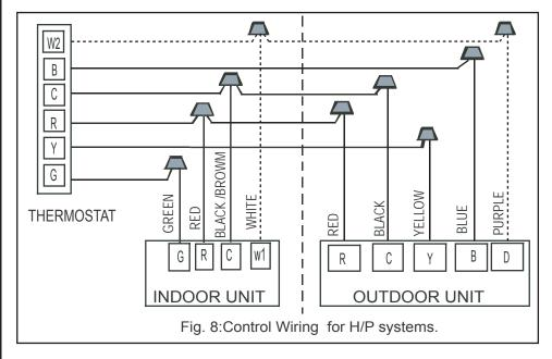
**Suggestion:** Thermostat choose CSW25B or Non-programmed eletrical thermostat series of Honeywell, such as TH 5220D. Broken lines means H/P system with electric heating. Wiring please refer to the Owner's Manual of the thermostat.
