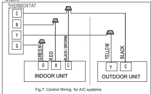
**Suggestion:** Thermostat choose CSW23B or Non-programmed eletrical thermostat series of Honeywell, such as TH 5220D. Wiring please refer to the Owner's Manual of the thermostat.
