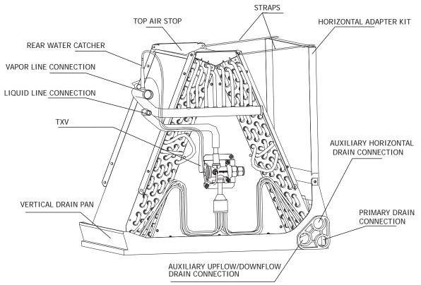
Fig.10 INDOOR COIL AND DRAIN PAN SET-UP
