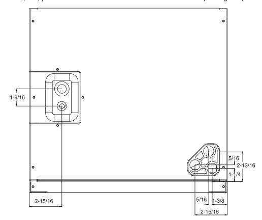
Fig.2 DIMENSIONS FOR FRONT CONNECT COIL
