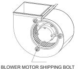
motor mount bolts) then check to see if wheel is secured to motor shaft before operating unit.
