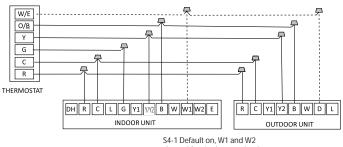
shorted for single stage Aux heat operation. Turn o to separate stages.
