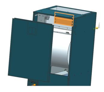
2. Remove the cover plate from the air handler.
