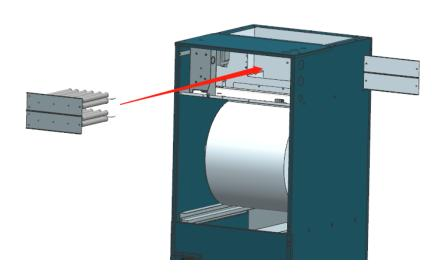
4. The heater installation completed.
