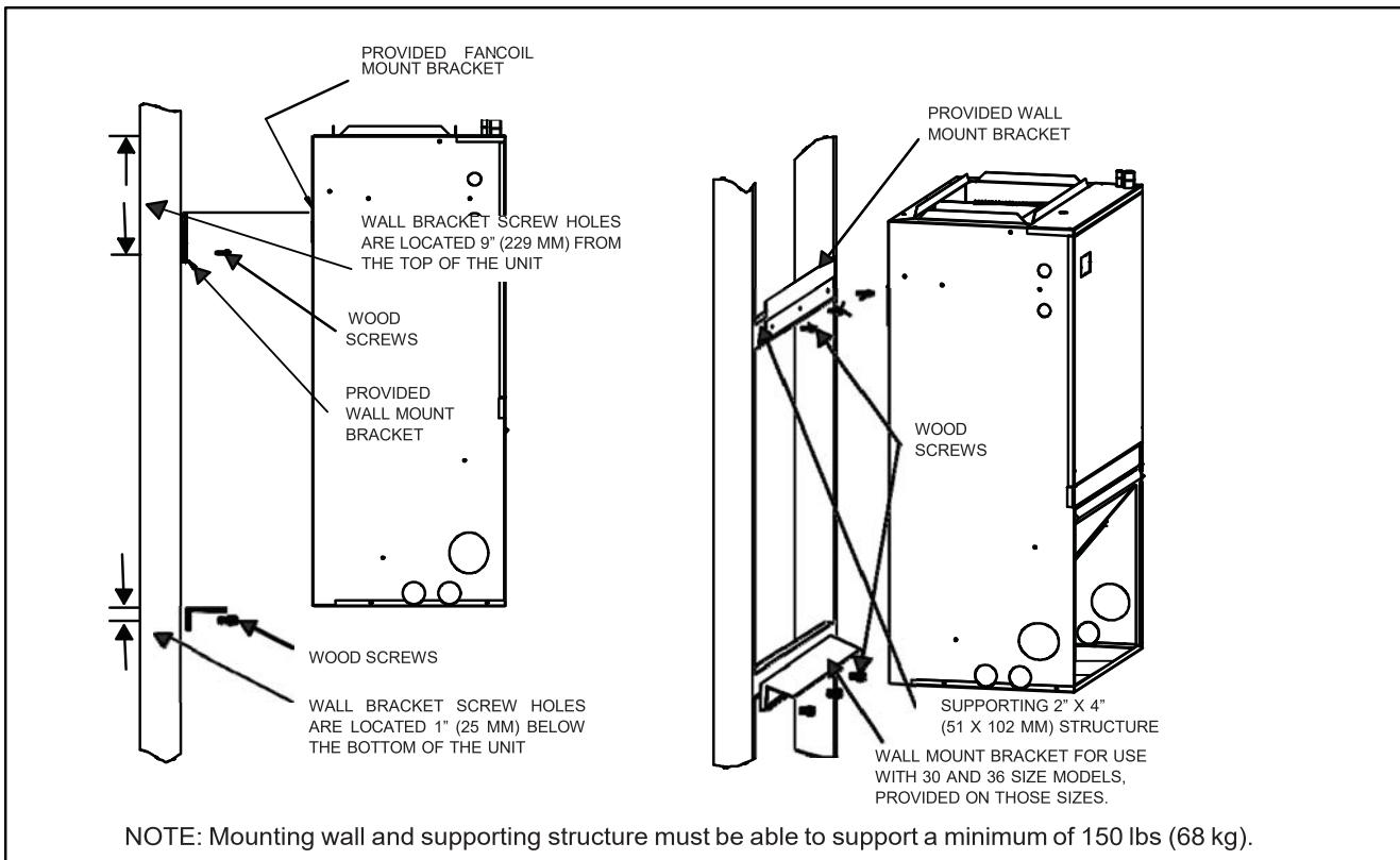
NOTE: Mounting wall and supporting structure must be able to support a minimum of 150 lbs (68 kg).
