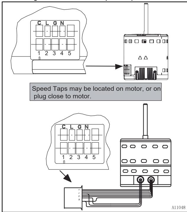
**Figure 10 - Wiring Layout PSC Motor disable time delay**
