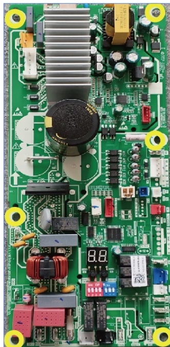
THE OUTDOOR CONTROL BOARD
