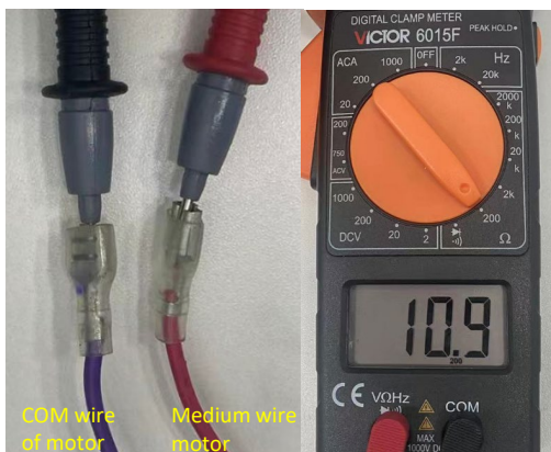
Example: Measure resistance of motor winding
