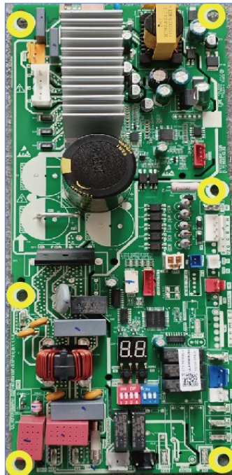
THE OUTDOOR CONTROL BOARD
