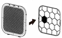
Separate the frame from the filter assembly.
