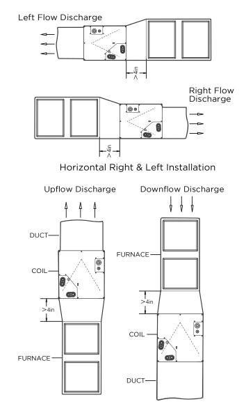
Vertical Upflow & Downflow Installation Adapter(s) Installation When Coil Overhangs Furnace
