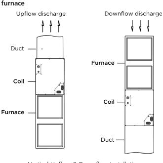
Model AC3-4860C-SG3 coil installation on
