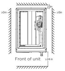
Top View of the indoor unit clearance (including air duct)
