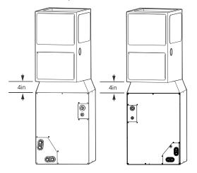
1. Set cased coil on supply duct opening.
