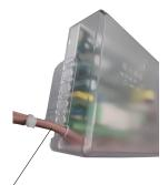
Use pliers to cut the upper cover, and cut the left position according to the diagram.
