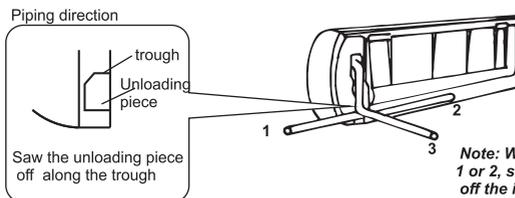
**Note:** When installing the pipe at the directions 1 or 2, saw the corresponding unloading piece off the indoor unit base.
