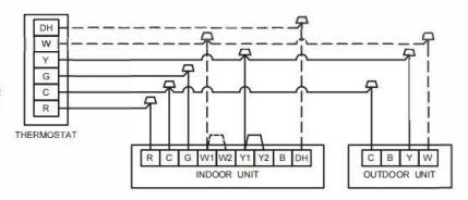
Wiring for 1H and 1C thermostat (no heat pump system model)
