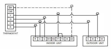
Wiring for 2H and 1C thermostat (no heat pump system model)
