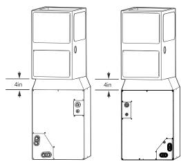
1. Set cased coil on supply duct opening.
