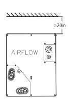
Front view of the indoor unit clearance (including air duct)
