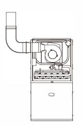
Fig. 6-12 Upflow Application-Vent Elbow Left
