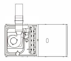
Fig. 6-10 Horizontal Left Application-Vent Elbow Up
