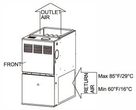
Fig. 3-1 Return Air Temperature
