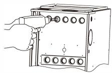
Fig. 14-3 Cleaning Heat Exchanger Cell
