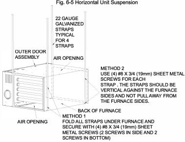
Fig. 6-6 Horizontal Suspension with Straps
