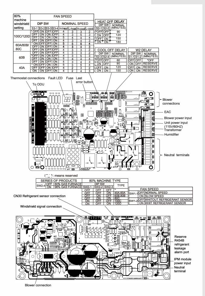
Fig. 9-2 Furnace Control
