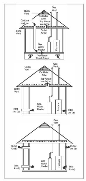
Fig. 7-3 Outside and Ambient Combustion Air
