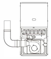
Fig. 6-8 Downflow Application- Vent Elbow Up then Left
