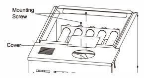
Fig . 7-1.B Cover the hole in the top panel when Combustion Air Inducer is rotated
