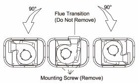
Fig. 7-1.A Combustion Air Inducer
