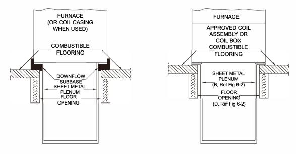
Fig. 6-3 Furnace, Plenum, and Subbase Installed on a Combustible Floor
