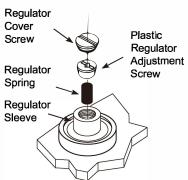
Fig. 10-1 Gas Valve and Regulator Adjustment
