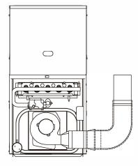
Fig. 6-9 Downflow Application- Vent Elbow Up then Right
