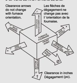
Vent Clearance to combustibles: For Single Wall vents 6 inches (6 po), For Type B-1 vent type 1 inch (1 po).
