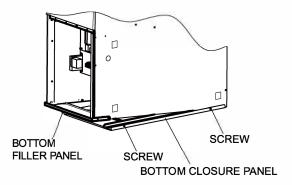
Fig. 6-1 Removing Bottom Closure Panel
