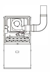
Fig. 6-14 Upflow Application-Vent Elbow Right
