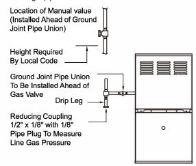
Fig. 8-2 Typical Gas Pipe Arrangement
