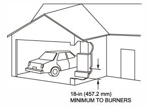
Fig. 5-1 Installation in a Garage
