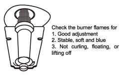
Fig. 11-1 Burner Flame
