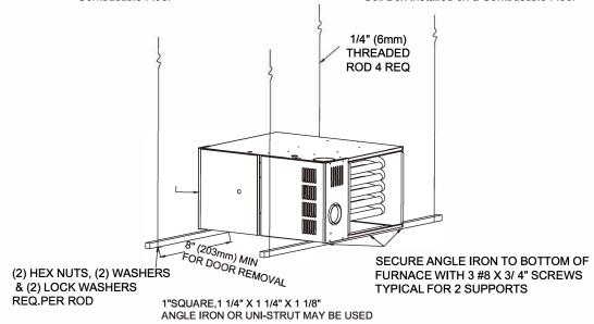
Fig. 6-5 Horizontal Unit Suspension
