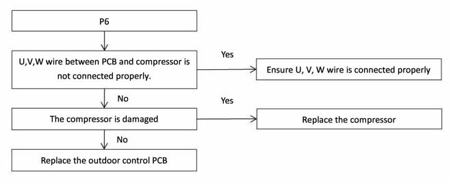
**Situation3:** P6 appears after the compressor has been running for a period of time.
