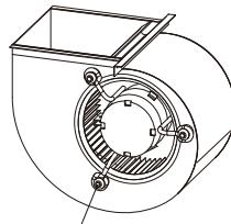
Make sure the blower motor support is tight (3-motor mount bolts), then check if wheel is secured to the motor shaft before operating the unit.
