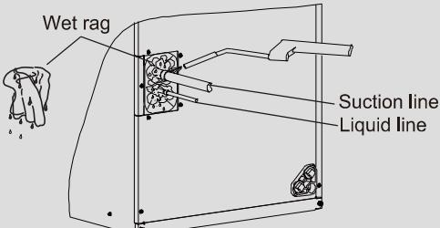
Fig.4-1 Piping connections
