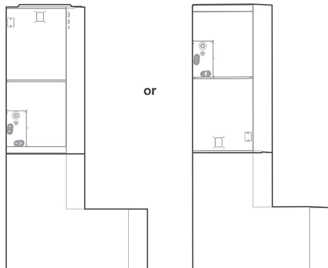
**Fixing instructions:** When installed vertically (upward or downward), the lower end of the air outlet needs to be connected to the L-shaped metal air duct and fastened by screws.
