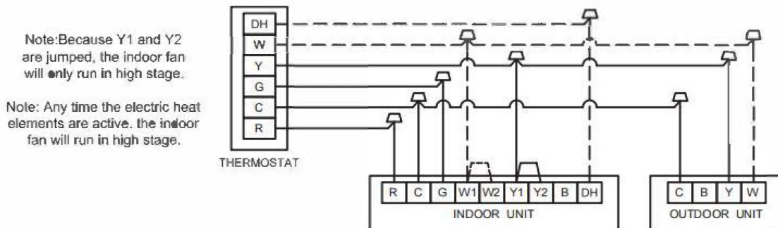
Wiring for 1H and 1C thermostat (no heat pump system model)
