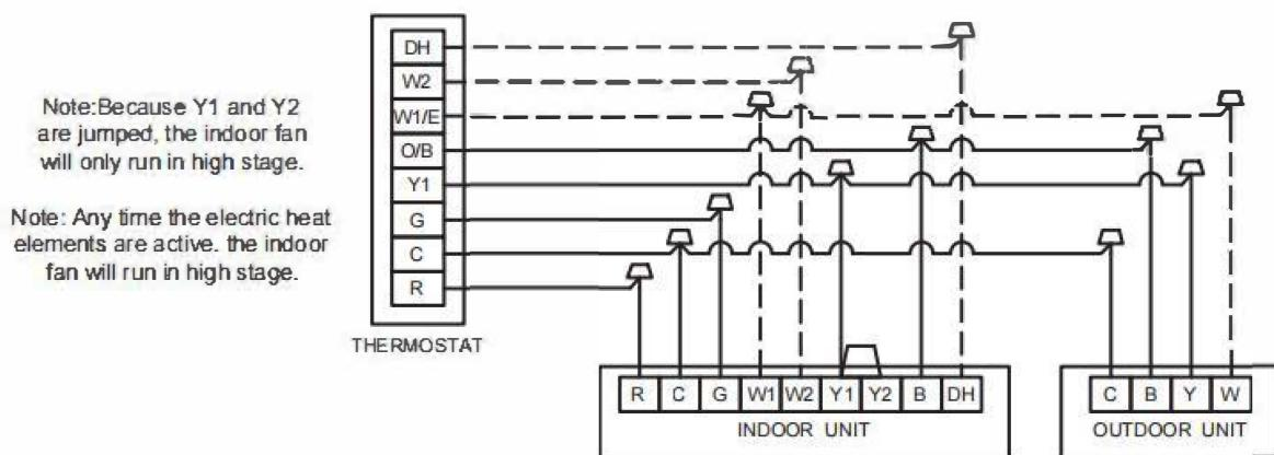
Note: Because Y1 and Y2 are jumped, the indoor fan will only run in high stage.
