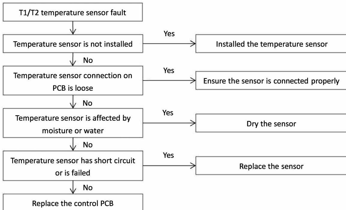
Note: Measure sensor resistance. If the resistance is too low, the sensor has short-circuited. If the resistance is not consistent with the sensor's resistance characteristics table, the sensor has failed.
