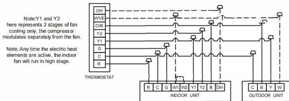
Note: Y1 and Y2 here represents 2 stages of fan cooling only, the compressor modulates separately from the fan.
