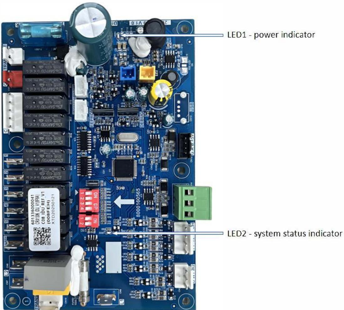
**Note:** In normal operation, LED1 and LED2 are steady on; when the system is standby, LED1 will be steady on, LED2 will flash slowly.
