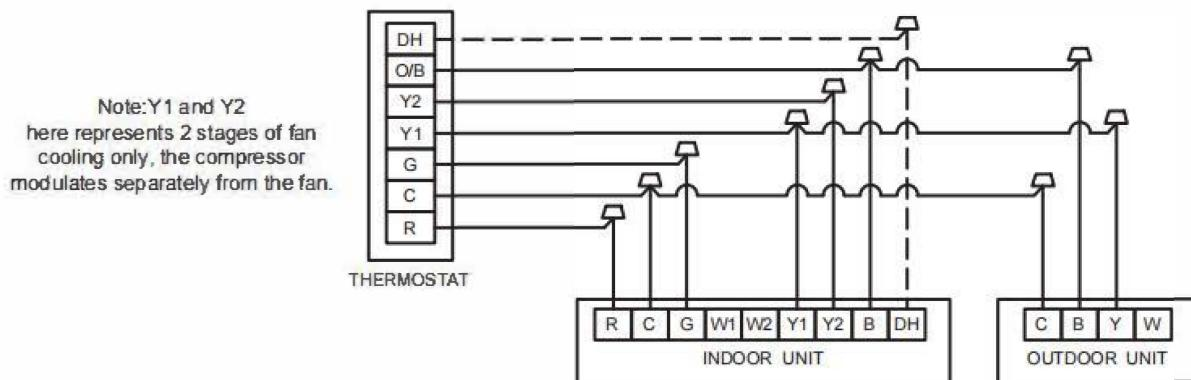
Note: Y1 and Y2 here represents 2 stages of fan cooling only, the compressor modulates separately from the fan.
