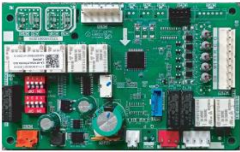
The control board for 60K
