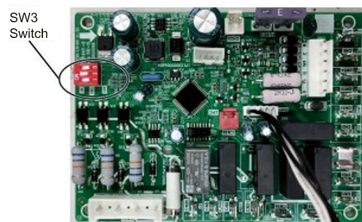
Fig.12-1 SW3 Switch Location in the main control Board (For reference only)
